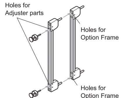
When using an Option Frame, insert the Adjuster Bolt following the direction of the arrow as shown above.
