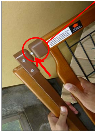
Figure 1. Locking Pin shown above does not lock properly.
