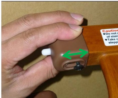
Figure 5. Determine which direction the Screw needs to be adjusted by sliding it using a phillips screwdriver. This will cause the Locking Pin to adjust itself to lock properly when the Door is closed.
