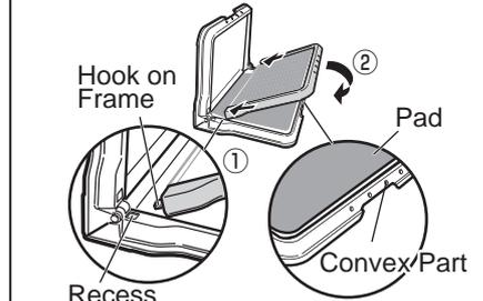
\* If the convex part of the tray is covered with the pad, the frame will come off easily.
